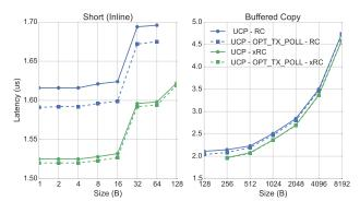
Fig. 10. RDMA write latency in UCP with optimization to avoid TX Polling
