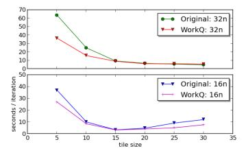
Fig. 4. Time per CCSD iteration for w3 aug-cc-pVDZ on ACISS versus tile size. The top row contains execution measurements on 32 nodes (384 MPI processes), and the bottom row contains measurements on 16 nodes (192 MPI processes).
