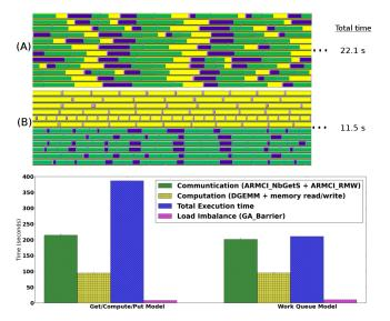
Fig. 1. (Top:) TAU trace of original code (A) compared to WorkQ (B) for a 192 MPI process job. Yellow is computation, purple is ARMCI\_Rmw (corresponding to Nxtval call), green is ARMCI\_NbGetS (corresponding to GA\_Get call), and pink is DGEMM. (Bottom:) Profile information comparing the two execution models for a larger 960 MPI process job. The work queue implementation accomplishes full overlap without sacrificing load balance.
