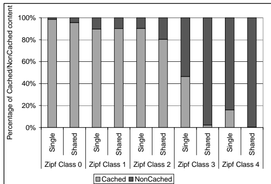
Fig. 8. Shared Data-Center Environment: Percentage of Cached and Non-Cached content for various workloads
